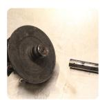
Insufficient Turbo lubrication
